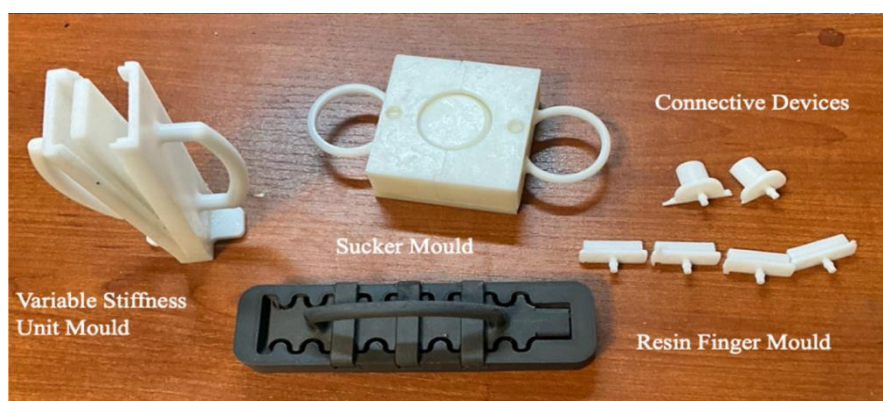
Figure. 7 3D-printed molds and connectives created by Finalist, 2024.
